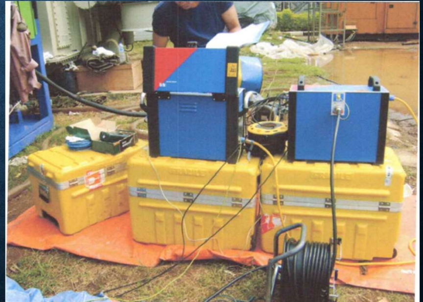
Characteristic and Tan Delta transformer testing
